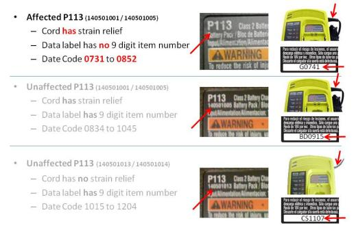
Photo 1 Ryobi Model P113 Dual Chemistry Charger Identification Label
