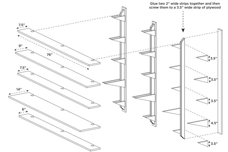
Screw triangular pieces of plywood to glued together strips of plywood to create shelf brackets
