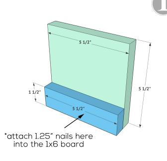
First, attach the 1x2 board tp the 1x6 board using wood glue and 1.25" brad nails. Make sure the 1x2 board is flush with one end of the 1x6 board.
