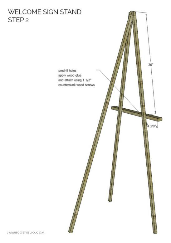
Step 3: Attach sign ledge using wood glue and 1 ½" countersunk wood screws.
