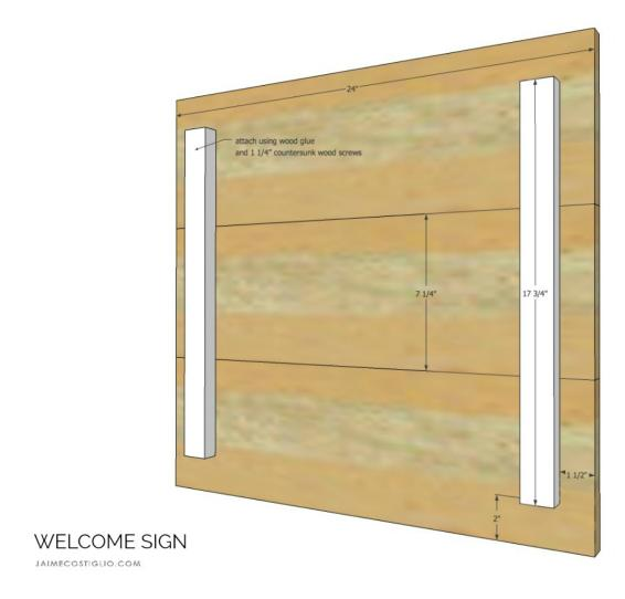
**Step 1:** Attach the cleats to the back of the sign boards using wood glue and countersunk 1  $\frac{1}{4}$ " wood screws.
