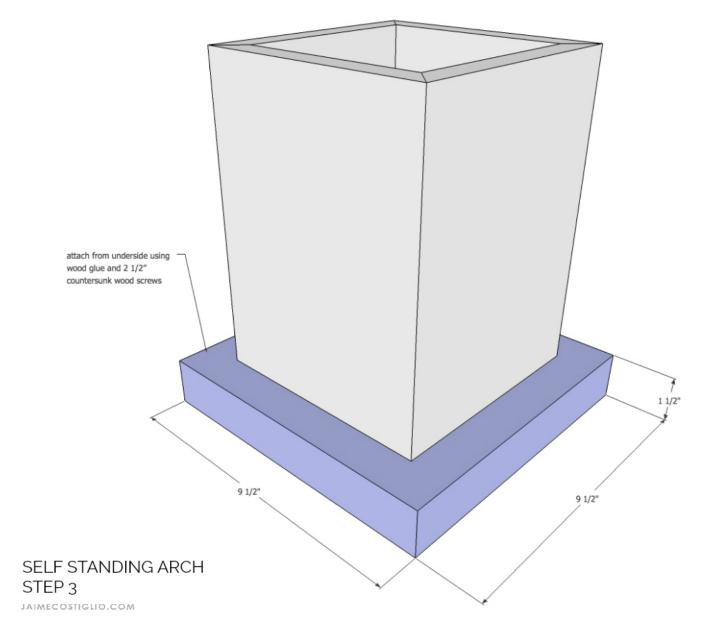
**Step 3:** Attach the base box to the base using wood glue and  $2\frac{1}{2}$ " countersunk wood screws from underneath.
