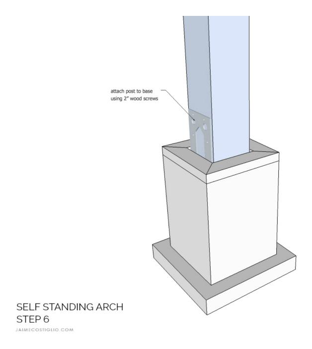
**Step 6:** Attach post to the hardware post base using 2" wood screws.
