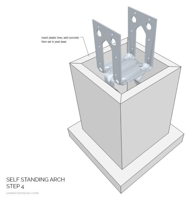
**Step 4:** Place a plastic bag into the base and then fill almost to the top with quik setting concrete. Insert the post base into the concrete keeping the hardware centered. Let dry.
