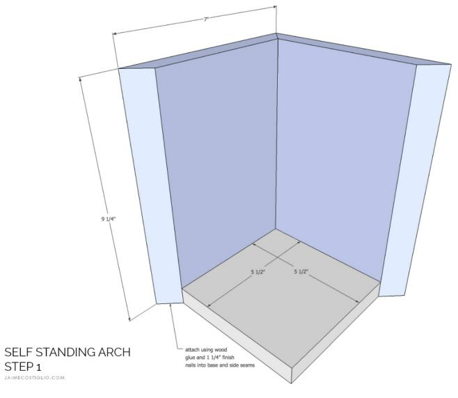
**Step 1:** Attach the base sides to the base bottom using wood glue and 1 1/4" finish nails.
