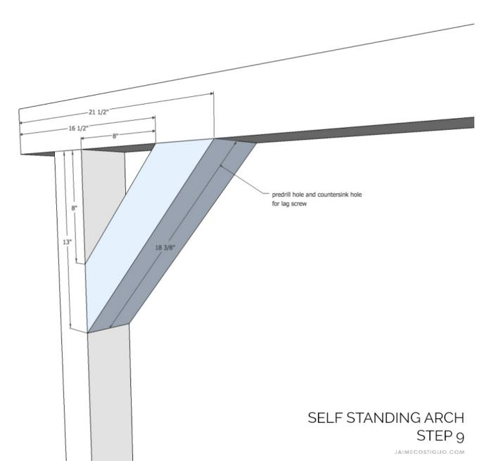
**Step 9:** Predrill holes for lag screws. Place corner supports in position and attach using lag screws (add a quick finish nail to hold while tightening screws).
