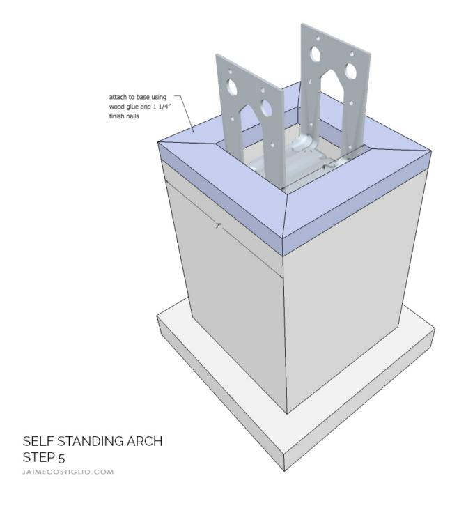
Step 5: Attach top trim to the base using wood glue and 1 ¼" finish nails.
