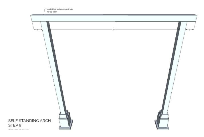
**Step 8:** Predrill holes for the lag screws and predrill countersink area for lag head. Place top beam in position and secure using lag screws.
