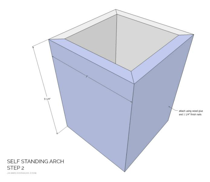
**Step 2:** Complete the base by attaching the other two sides to the each other and the base using wood glue and  $1\frac{1}{4}$ " finish nails.
