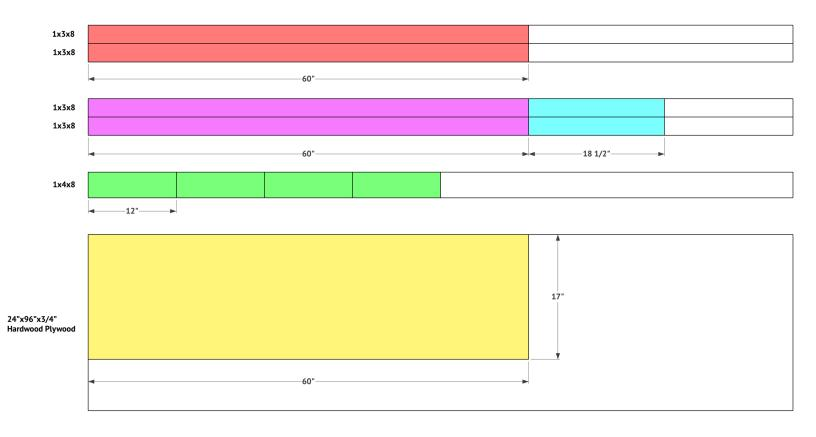
Note: Before cutting the hardwood plywood to size, lay the mirrors and wood down on the plywood to make sure it is a perfect fit.
