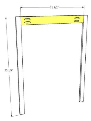
Drill  $\frac{3}{4}$ " pocket holes into each end of the 1x4 piece. Glue and clamp the 1x2 pieces to each side, flush at the top. Attach with 1  $\frac{1}{4}$ " pocket screws.
