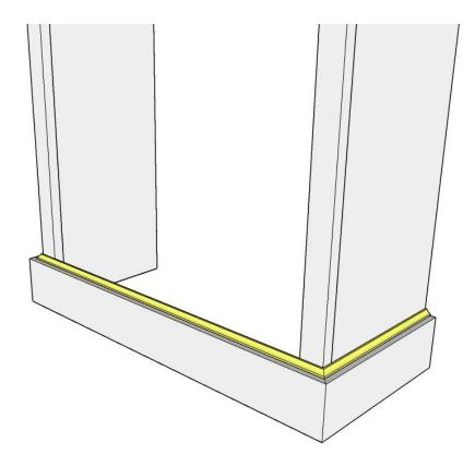
Measure and cut to size cove moulding with 45 degree angle on one end for sides and 45 degree angles on each end for front. Attach with wood glue and ¾" brad nails.
