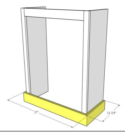
Measure and cut to size 1x4 pine boards for bottom moulding w/ 45 degree angle on one end for sides and 45 degree angles on each end for front.. Attach with wood glue and  $1 \frac{1}{4}$ " brad nails.
