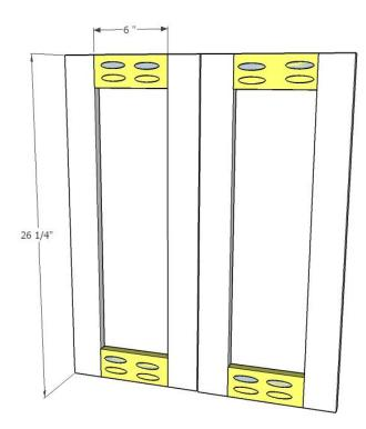
Cut oak cabinet face frames to size. Drill  $\frac{3}{4}$ " pocket holes into 6" cabinet rails. Build cabinet doors with wood glue and 1  $\frac{1}{4}$ " fine thread pocket screws. Finish as desired with paint or stain.
