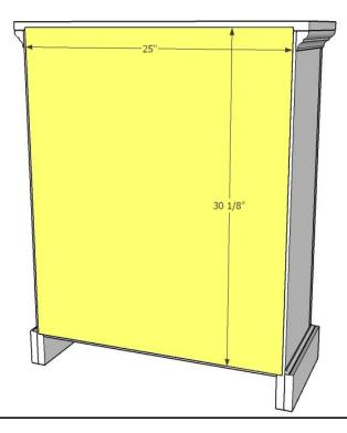
Cut hardboard backing to size and attach with ¾" narrow crown staples.
