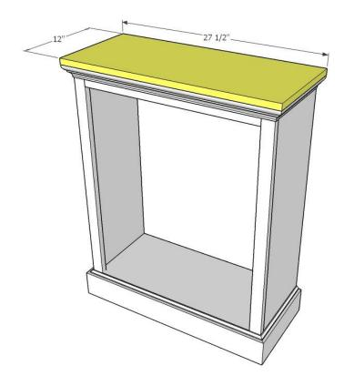
Glue veneer edge banding to sides and front of cabinet top. Attach cabinet top with approx  $\frac{1}{4}$ " overhang on sides and front, with wood glue and  $\frac{1}{4}$ " pocket screws.
