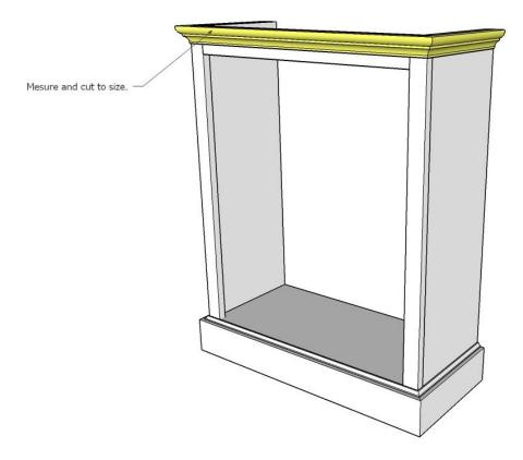
Measure and cut to size the top moulding with 45 degree angles on one end of sides and 45 degree angles on each end of front piece. Attach with wood glue and  $1 \frac{1}{4}$ " brad nails, flush with the top of the cabinet.
