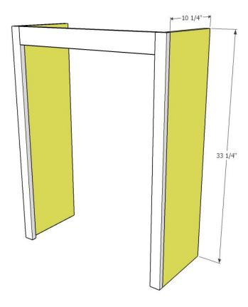
Drill  $\frac{3}{4}$ " pocket holes into top ends of cabinet sides. Line up the  $\frac{3}{4}$ " plywood sides flush with the outside edge of the 1x2 face frame. Glue and clamp into place. Attach with 1  $\frac{1}{4}$ " brad nails.
