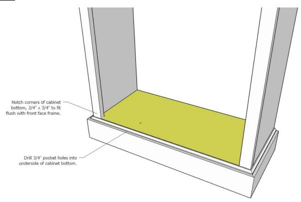
Notch the front of the cabinet bottom with  $\frac{3}{4}$ " notches to fit around face frame. Drill  $\frac{3}{4}$ " pocket holes into the underside. Flip cabinet onto back and set bottom flush with the top of the cove moulding. Attach with  $1\frac{1}{4}$ " pocket screws.
