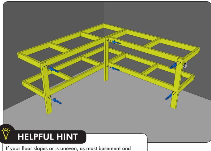
If your floor slopes or is uneven, as most basement and garage floors do, you can easily add shims under the legs to level out your shelves.
