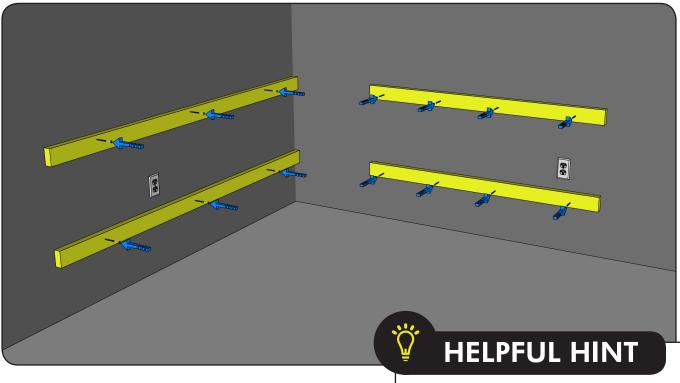
Remember to leave a space of 24" between the 60" 2x4 and the wall perpendicular to it, as this space is meant for more support material in later steps.
