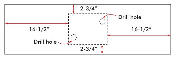
Drill two holes inside opposite sides of the rectangle you've just drawn. Use the holes as the starting point to cut out the opening with a jig saw.
