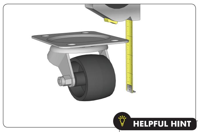
To get both side walls and middle divider from one half of plywood sheet, plan on using caster wheels at least 2-1/2" or taller.
